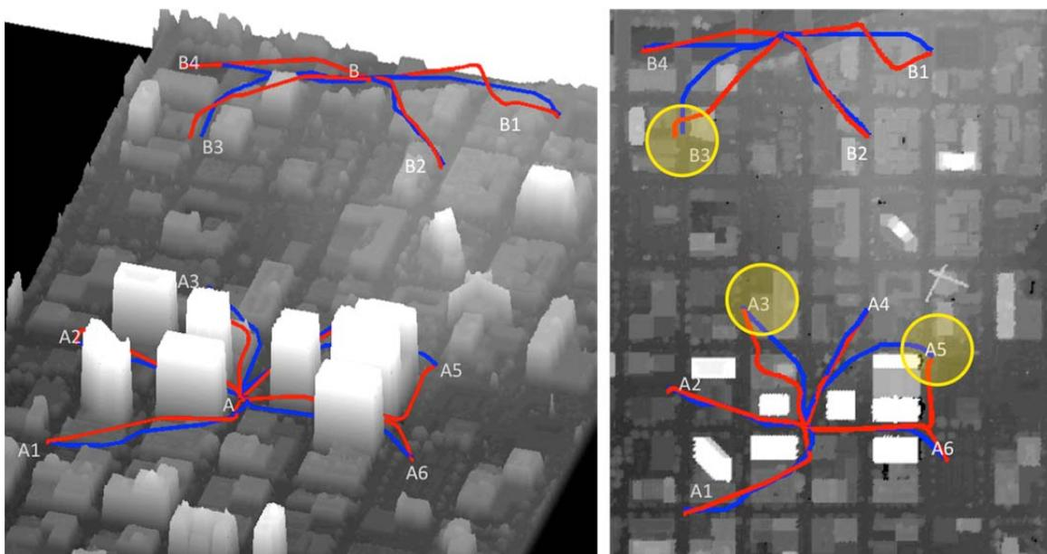
Figure 2: Trajectories of two sets of urban test case scenarios ("A" and "B"). Results are shown for the benchmark's baseline (blue) and MiPIEx (red) at  $d_{\text{sample}}=20$  m that was configured with a LIDAR obstacle sensor  $d_{\text{range}}=70$  m.
