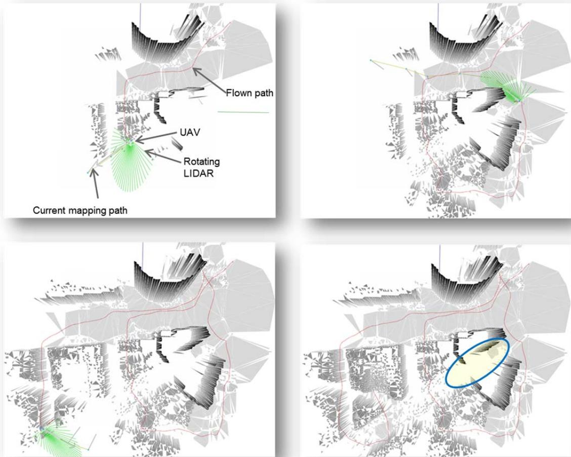
Figure 3: Top view of the exploration progress (from upper left to lower right). Example scenario shows city of Berlin at Potsdamer Platz: The rotorcraft decides for each temporary waypoint based on a cost-modified roadmap.
